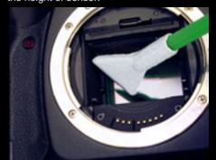
Lift off sensor, rotate swab width to width of sensor and remove.
