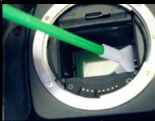
Contact sensor so that swab width is edge to edge of the height of sensor.
