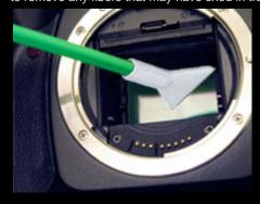
Insert swab width wise to the width of the sensor. Rotate once inside chamber.
